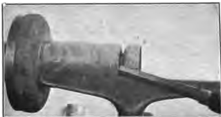
Fig. 110. Cover, with Knob Being Cut Off.
